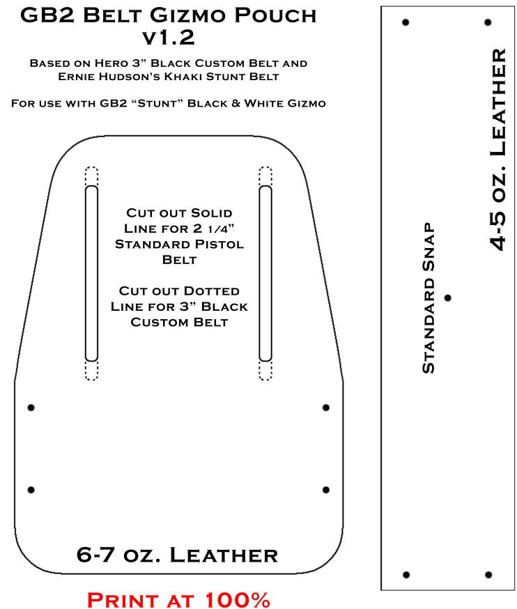
Assemble with 3/8" Head Rivets (Size Medium) through the 4 holes on both portions.
